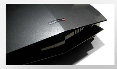
A state-of-the-art projector that integrates the latest technologies available on the market such as 1080p resolution (1920x1080 3-LCOS engine) and HDMI 1.3 connection inside a futuristic chassis designed by Pineau & Le Porcher.
