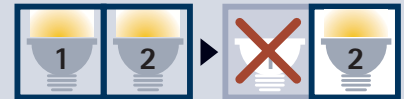
With the two lamp system, the second, intact lamp is used if one lamp fails.
