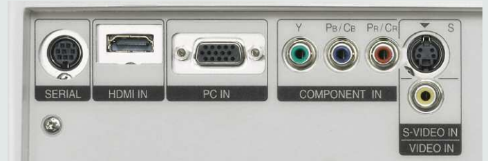
A variety of terminals including HDMI input
