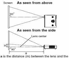
a is the distance (m) between the lens and the screen, and corresponds to a range of 1.20 m to 10.00 m. **H** is the height from the image bottom to the center of the lens.
