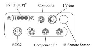
\*SCART RGB & Component I/P (via supplied adapter)
