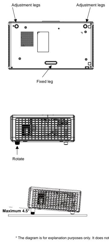
The diagram on the left shows the underside of the unit.
