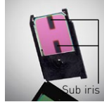
The sub iris cuts light leakage.
