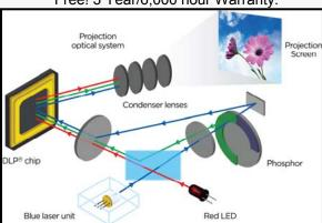
By combining a laser, a fluorescent element and an LED Casio has created an original mercury-free hybrid light source capable of generating high brightness. Casio has achieved high brightness output of green light, which until now, has been considered difficult with conventional semiconductor light sources, by efficiently converting blue laser light into green light using a fluorescent element.
