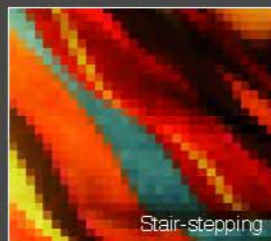
Angle Motion Compensation removes stair-stepping on moving diagonal lines.
