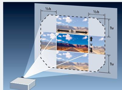
*The projected image can be adjusted a half screen to the right or left as well as a full screen up or down.*
