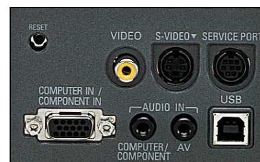
PLC-SW30 Terminal Input Panel
