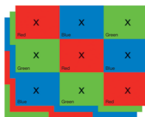
Colour Light Output uses 3 sets of a nine-point grid to measure the primary colours – red, green and blue
