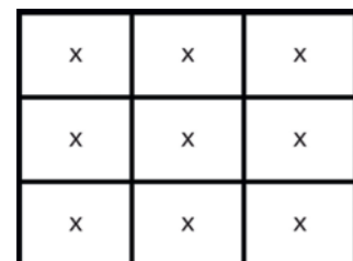
Brightness (or white light output) measures the total amount of white light projected in lumens on a nine-point grid
