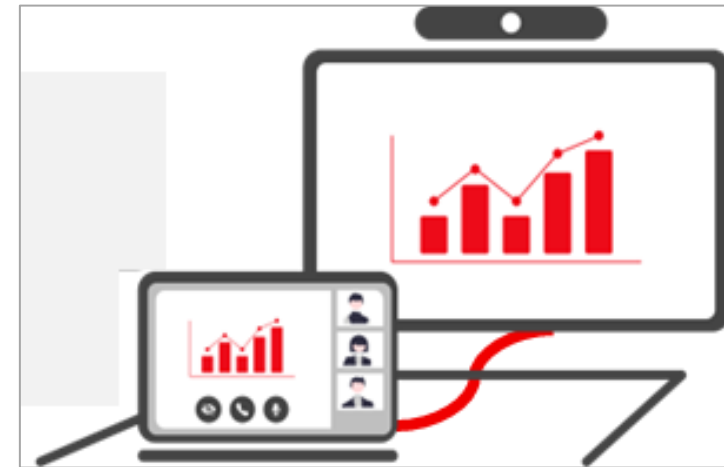
Cabled connection from PC to ClickShare if Wi-Fi is restricted or if you need native 4K.
